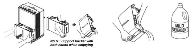
NOTE: When the bucket is full or removed from the machine, the compressor will turn off, but the fan will continue to run for a few minutes. This is completely normal. The dehumidifier will not be removing moisture from the air at this time.
